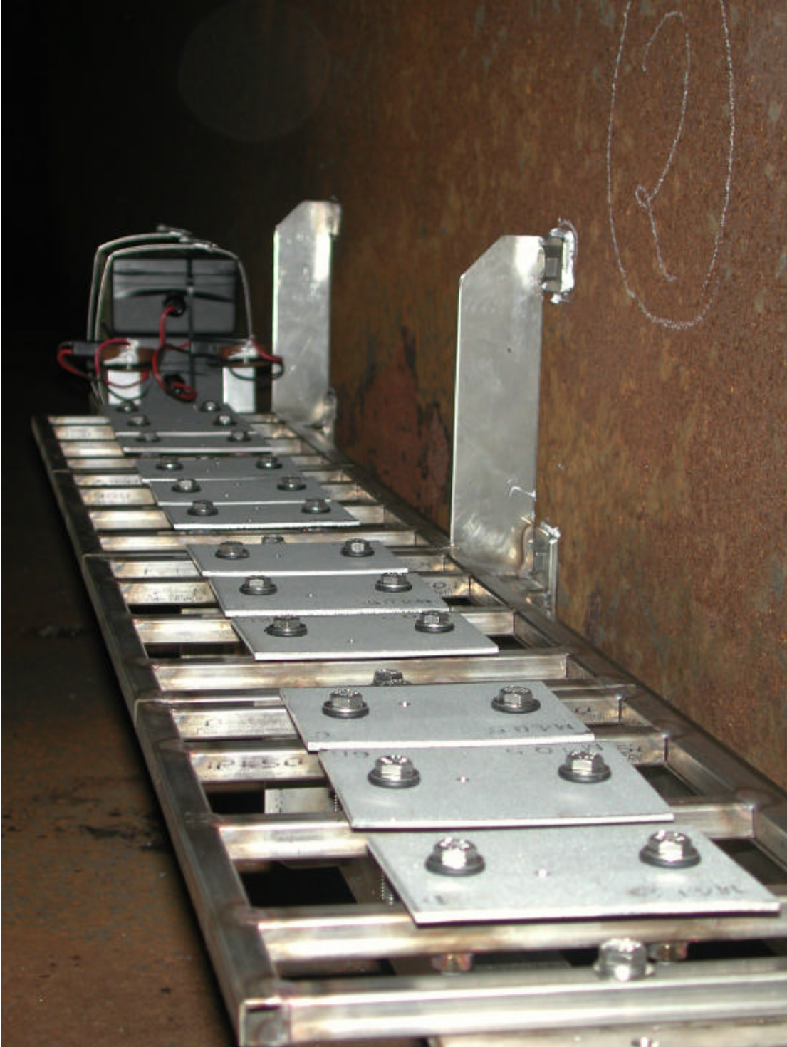
Photograph 17: Specimen Rack 2 (end view), installed at location 3DN above right lane of I-390 S.
