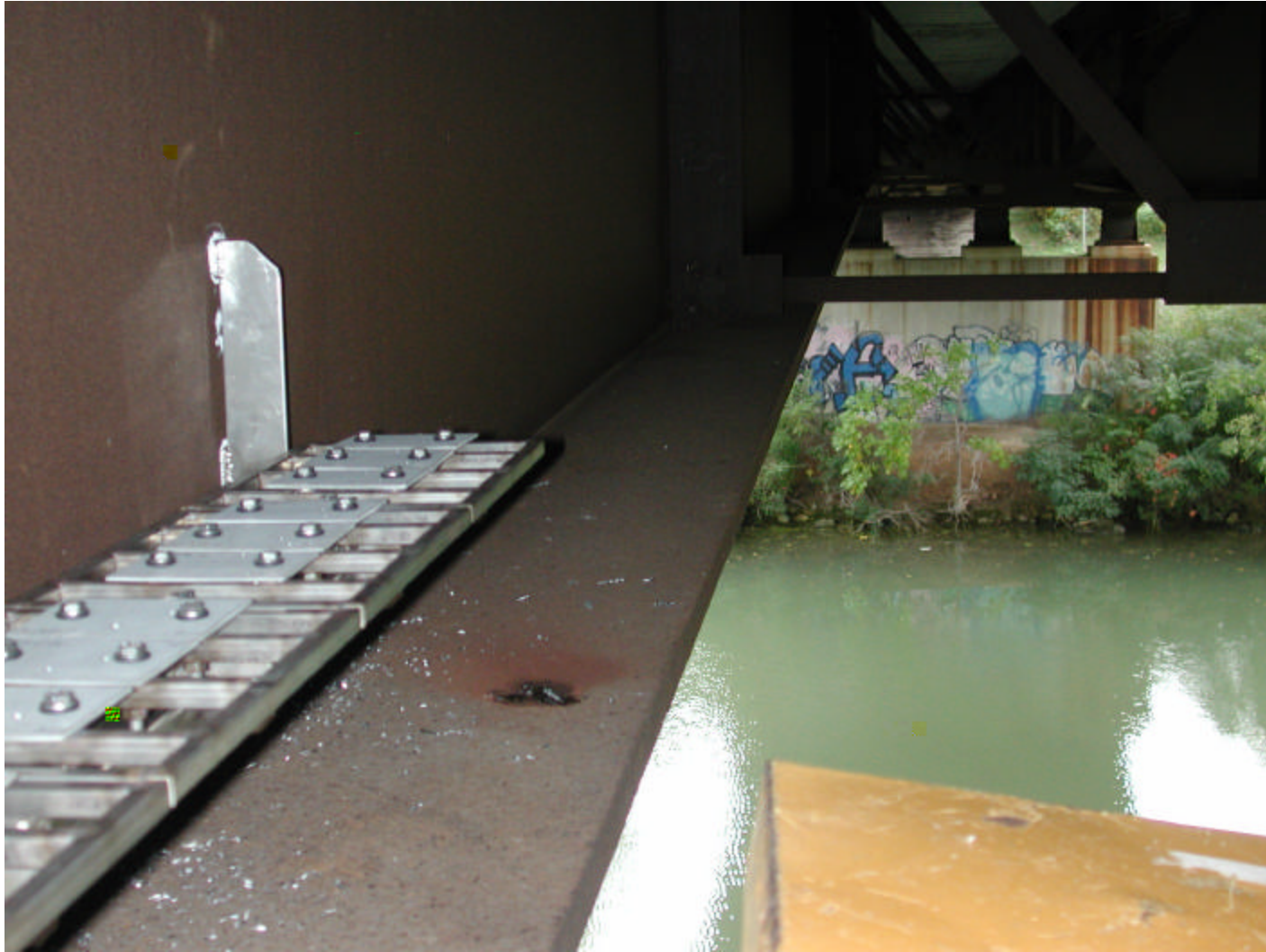
Photograph 22: Specimen Rack 3 installed above the jogging path at the edge of the Erie Canal.
