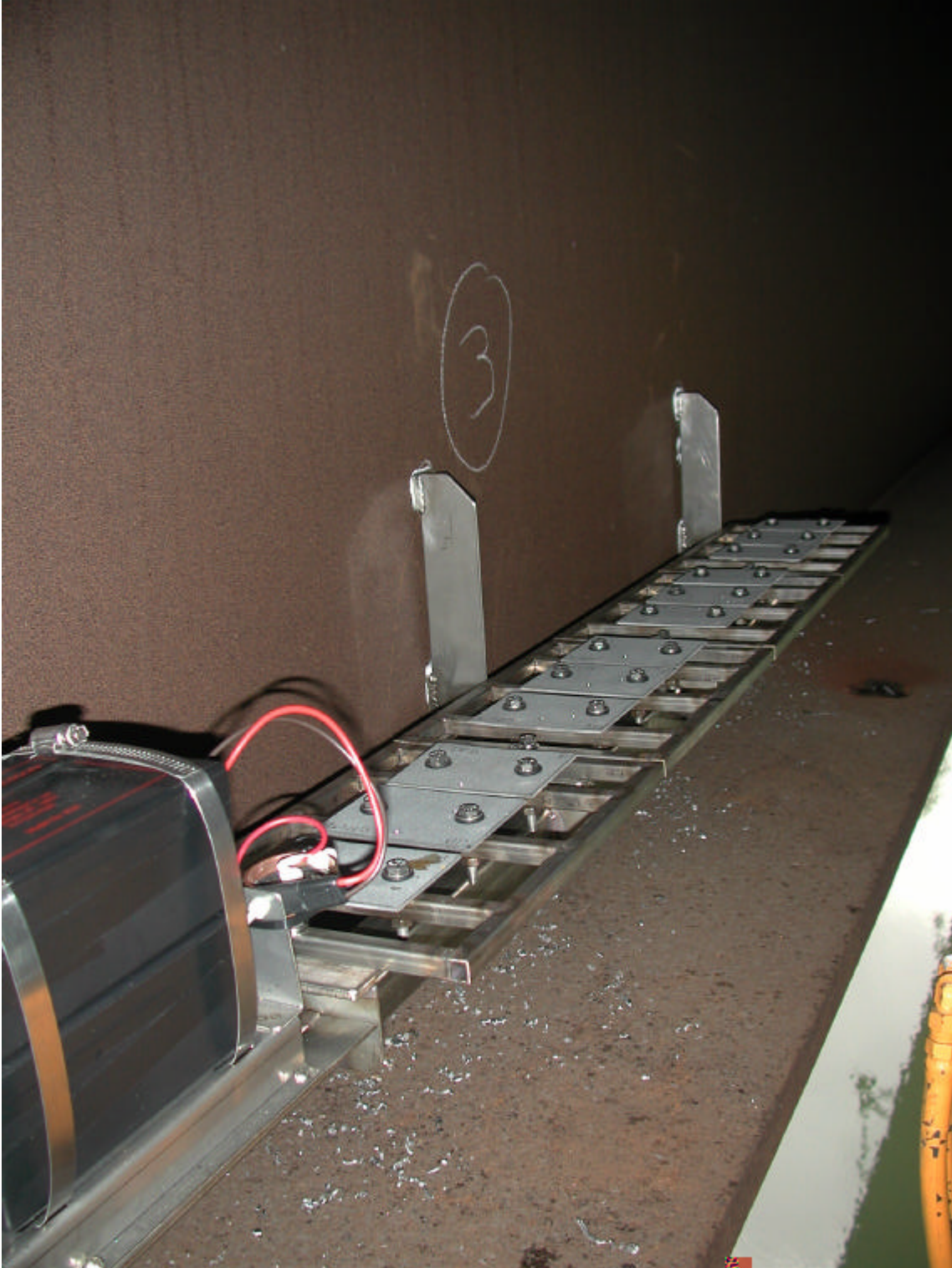
Photograph 20: Specimen Rack 3 installed at location 3MN at the East abutment. Thickness measurement positions are visible on the flange below each end of the rack.
