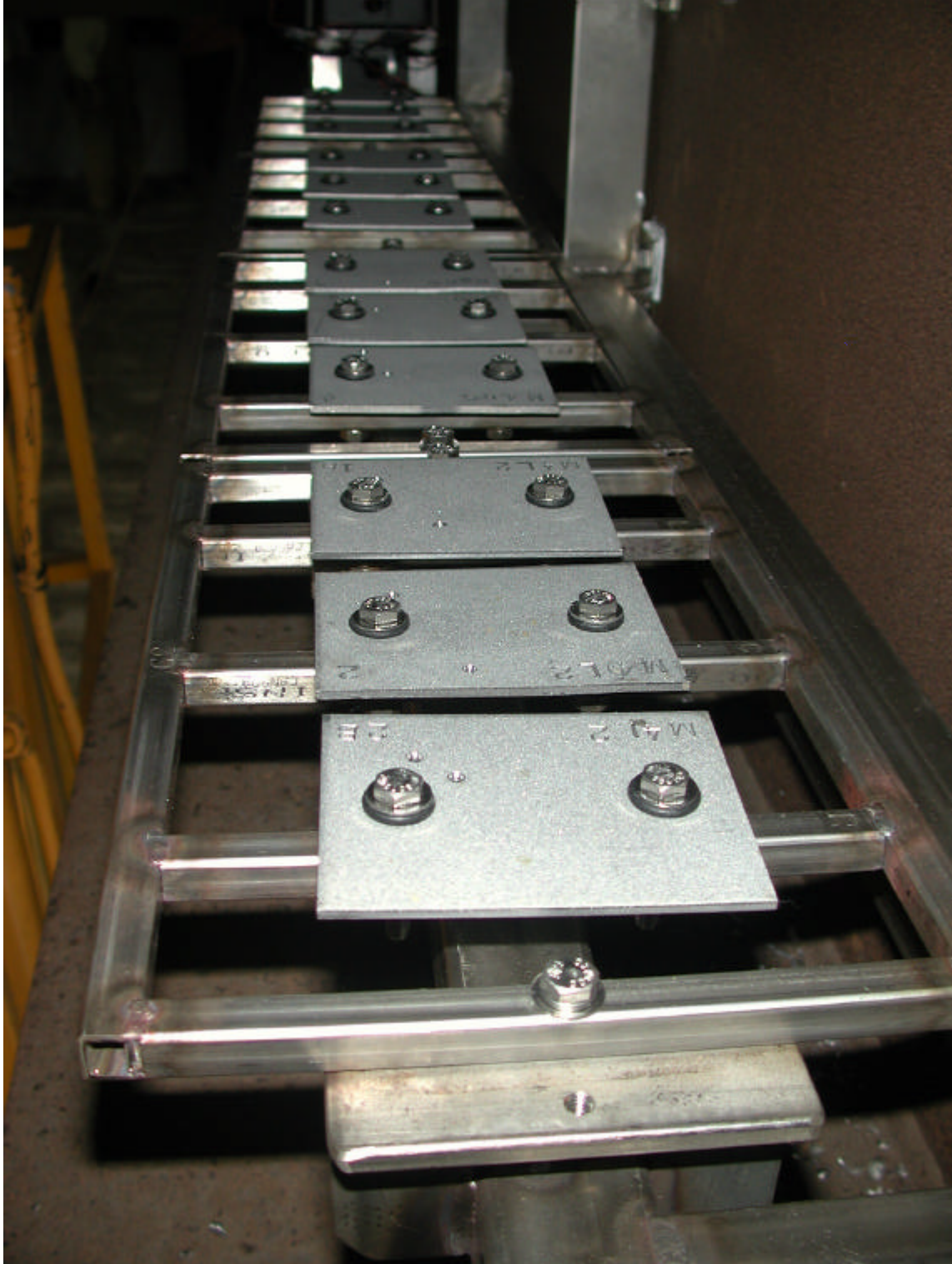
Photograph 21: Specimen Rack 3 (end view) installed at location 3MN above the jogging path at the east abutment.
